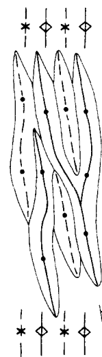
Fig. 9. Schematic development of periclinal folds of en-echelon and branching forms. Heavy lines are antiformal axes; broken lines are synformal axes. The orientation of the initial fold axes is given at the top and bottom. Initiation sites are shown by dots. Fine lines show the limit of final fold geometry. \theta is the axial migration angle ( = 10^\circ ).
